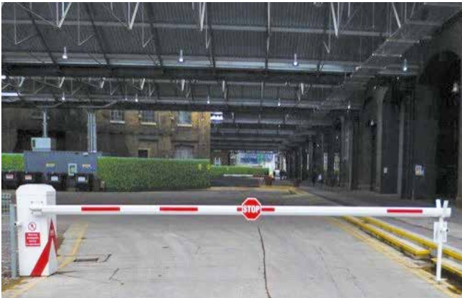
Fig 9. Typical powered lifting pole barrier
