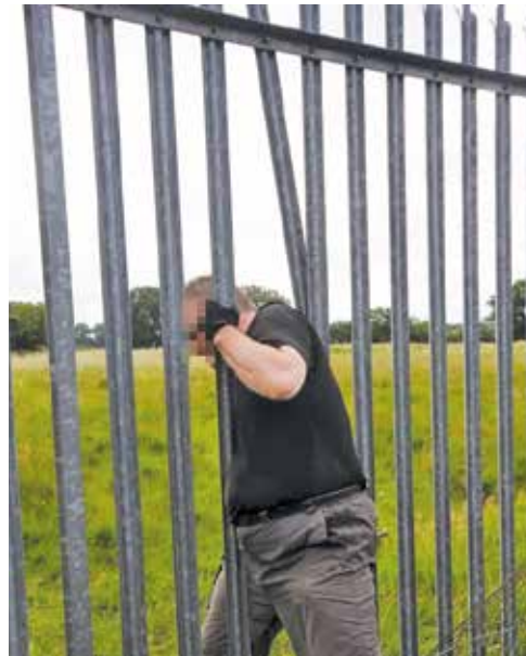
Fig 5. Palisade fence 'pendulum' attack
