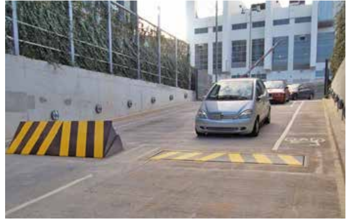
Fig 10. Rising step barriers (raised left, lowered right)
