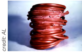
Figure 2: Wound extension cable showing overheating
