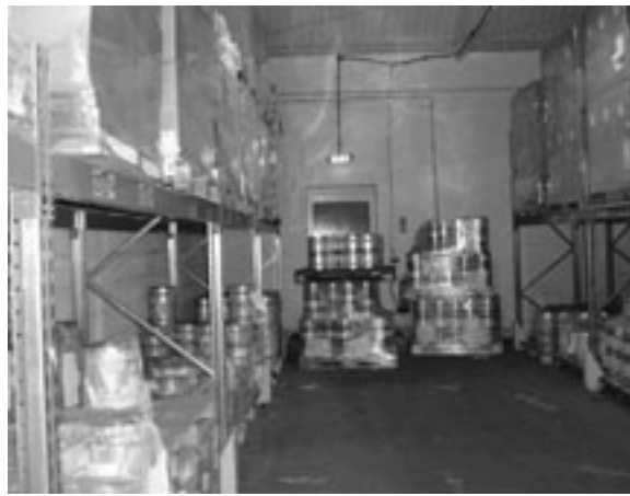
Poor housekeeping can lead to blocked escape routes
