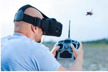
**Piloting a drone using VR goggles conflicts with the legal requirement to keep the drone in sight**
