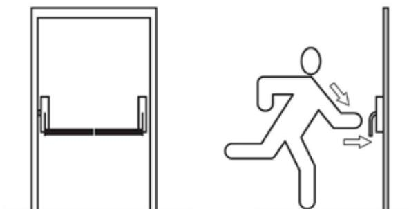
Fig 1: BS EN 1125 device with push-bar operation
