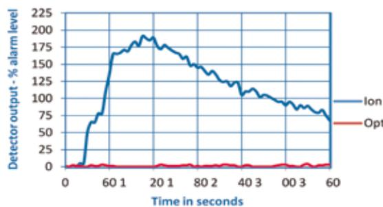
**Figure 1. Response of ion-chamber and optical detectors to a dusty gas heater**
