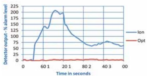
**Figure 2. Response of ion-chamber and optical detectors to soldering a plumbing joint**
